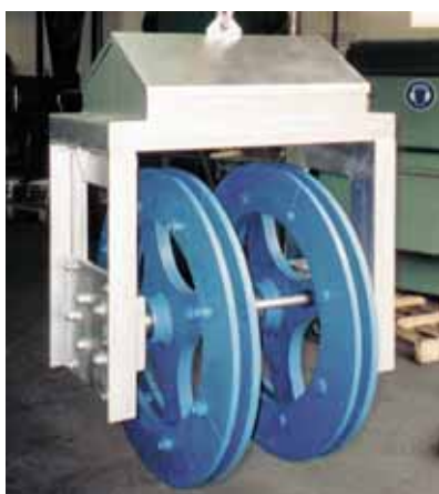
Figure 68: Pre-assembled HEKO Return and Tensioning unit, complete with segmented rims and spacer bars.
