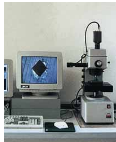
Figure 9: Automatic hardness tester (Protocolling of hardness values and hardness curve)
